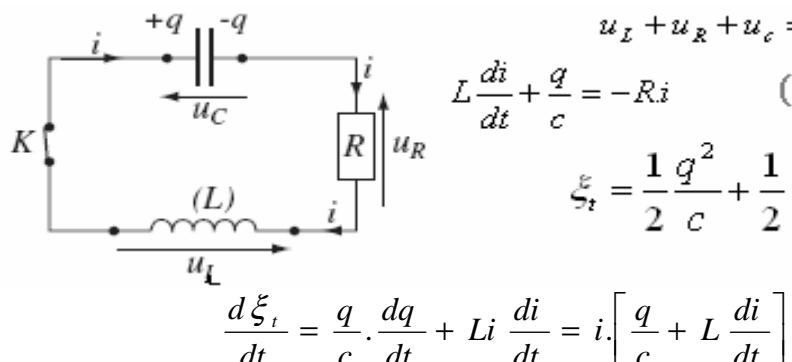
$$\frac{d\mathcal{E}_t}{dt} = \frac{q}{c} \cdot \frac{dq}{dt} + L i \frac{di}{dt} = i \left[ \frac{q}{c} + L \frac{di}{dt} \right] \quad \text{إذن :}$$
